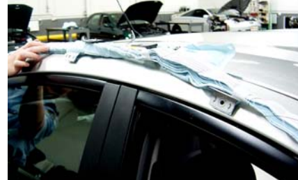
Side impact curtain and gas cylinder assembly shown laid in position over the top of the actual installation in the roof lining.
