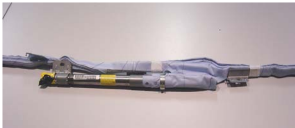
Side impact curtain and gas cylinder assembly shown laid in position over the top of the actual installation in the roof lining.
