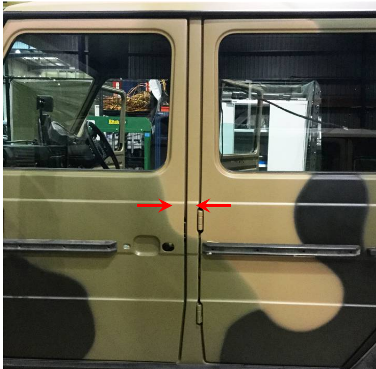
Figure 5: Small door gap
