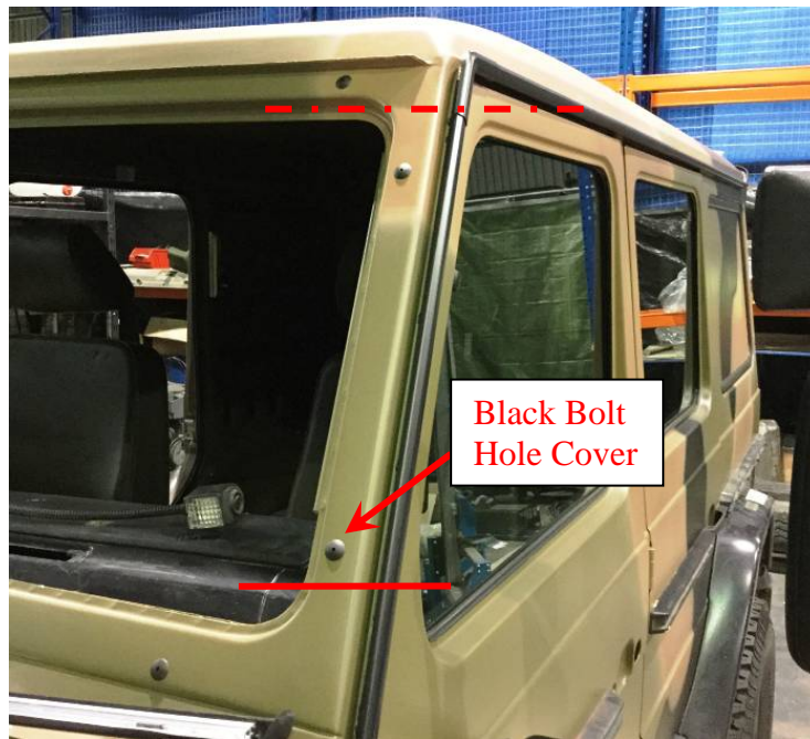
Figure 7: Recommended A pillar cutting points
