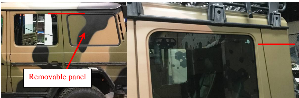
Figure 11: Station Wagon C pillar Figure 12: 6x6 Dual Cab C pillar
