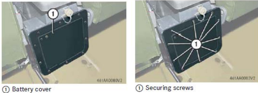
Figure 3: Centre Console Battery location
