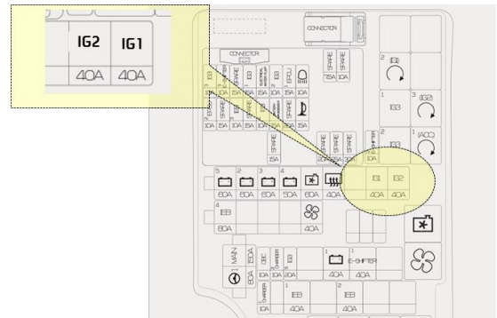
motor compartment fuse box
