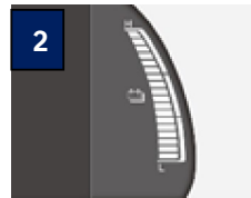
2 SOC (High Voltage battery). The gauge indicates the charge state of the high voltage battery.
