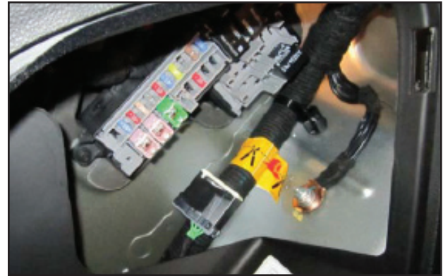
12V Battery Positive Cable located in rear compartment behind fuse panel door
