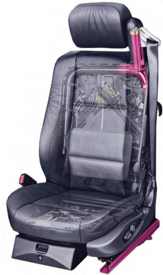
Seat-integrated seat belt system (SGS)
