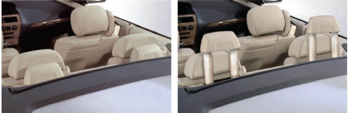
Rollover protection device for the 6 Series E64 in normal position and triggered (right)
