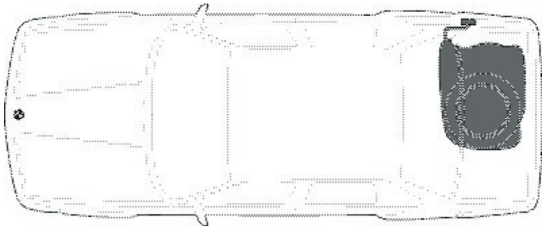
Installation drawing, fuel tank
