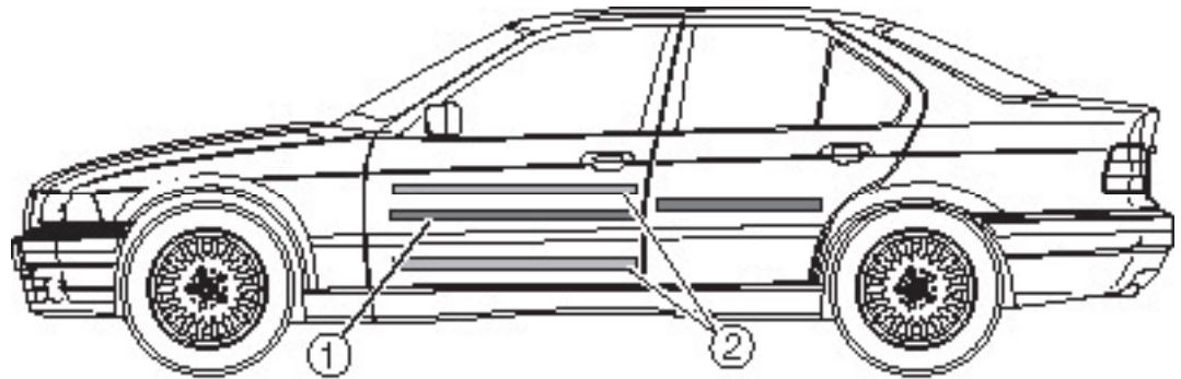
Installation drawing, side-impact protection, horizontal
