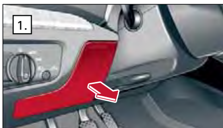
Fuse box – left-hand drive (steering wheel left)
