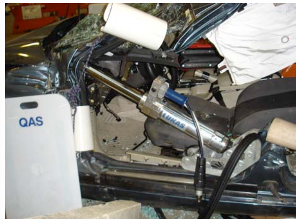
Fig 3: Modern NCT version B pillar cut higher for purchase and to effect ramming option.
