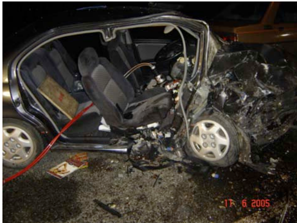
Fig 1. Case study crew forced to centre dash roll instead of working from the 100% option of the B pillar with rear door in place.
