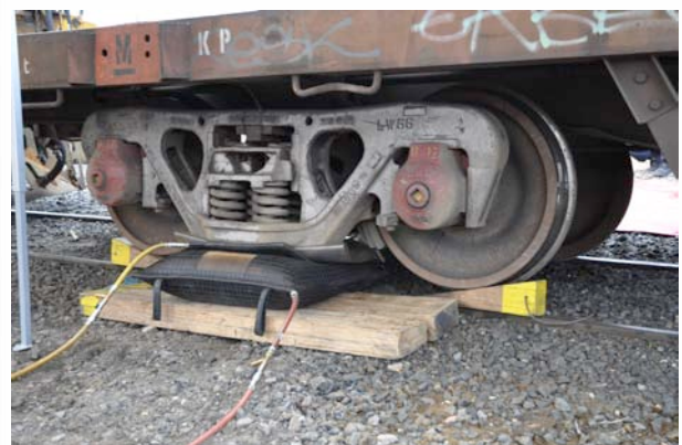
Bogie lift with wedges under the wheels as stabilisation
